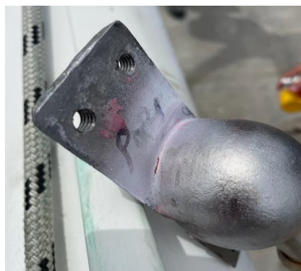
Port ball tang cracked so replaced
